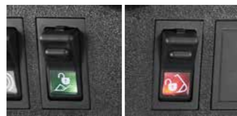
Safety Switch (Loader) Safety Switch (Backhoe)
