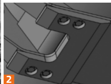
2 CHANGEABLE BOTTOM PLATES Operator can change wear plate easily
