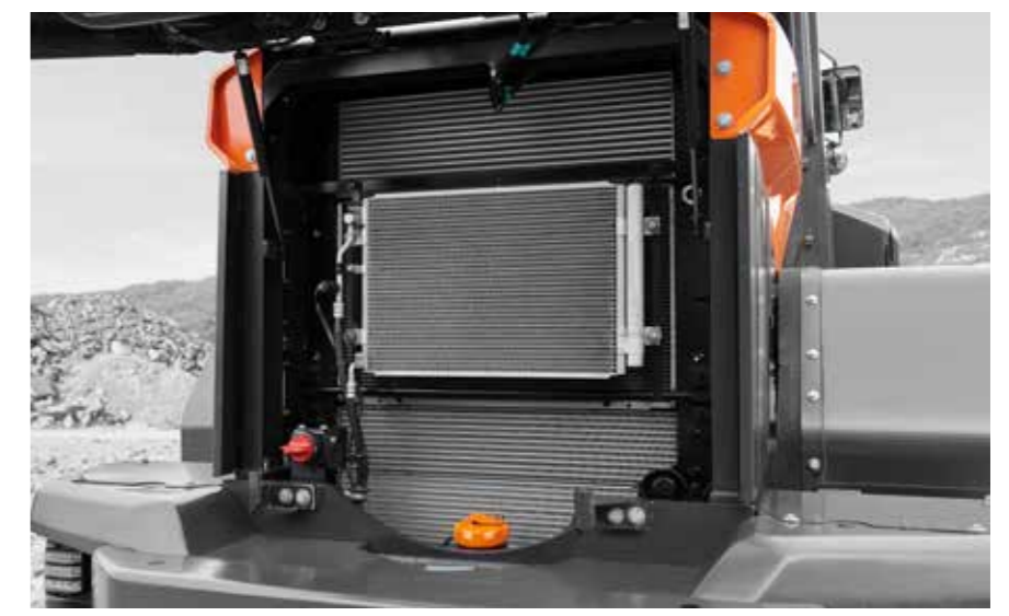
SINGLE LAYER COOLING MODULE RADIATOR Applied Single layer cooling module structure. Simple structure made easy for cleaning.
